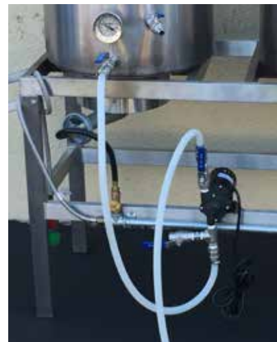
Hoses set up for transfer to fermenter *Shown on a Low Rider System
