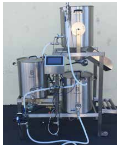
Hoses set up for Sparging
