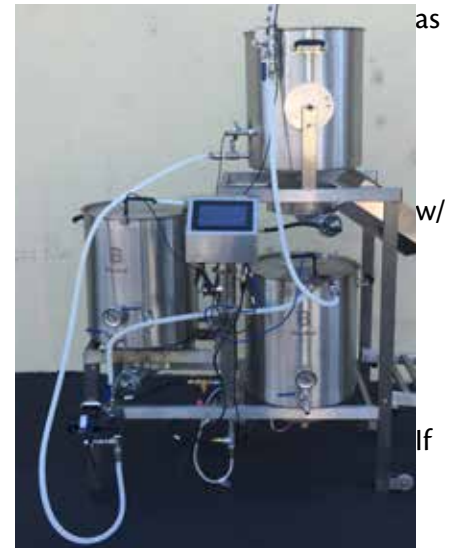
Hoses set up for Mash Recirculation
