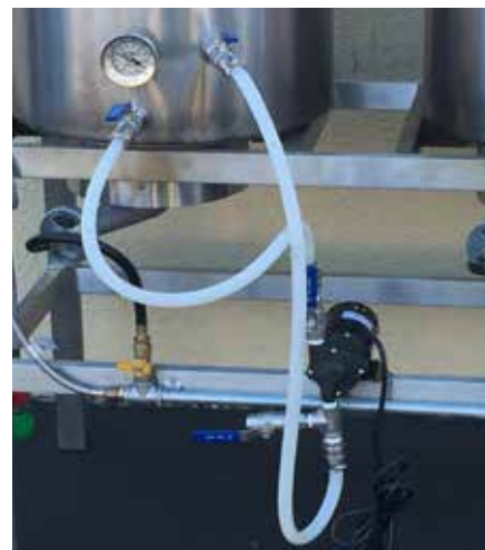
Hoses set up for Whirlpool *Shown on a Low Rider System
