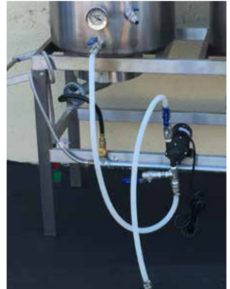
Hoses set up for transfer to fermenter *Shown on a Low Rider System
