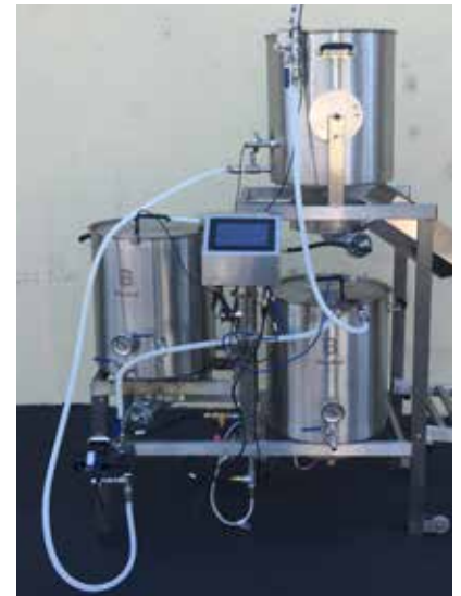
Hoses set up for Mash Recirculation
