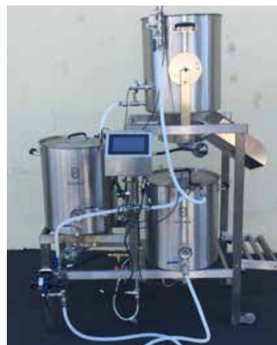
Hoses set up for Sparging
