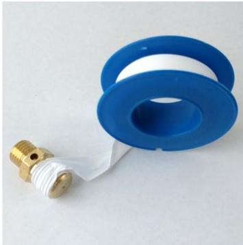
3. Use Teflon tap to cover the thread of the ball valve then screw it into the side of the still body. See pictures to right. No need to use a spanner. Just finger tight is fine here. Over tightening might damage the thread.
