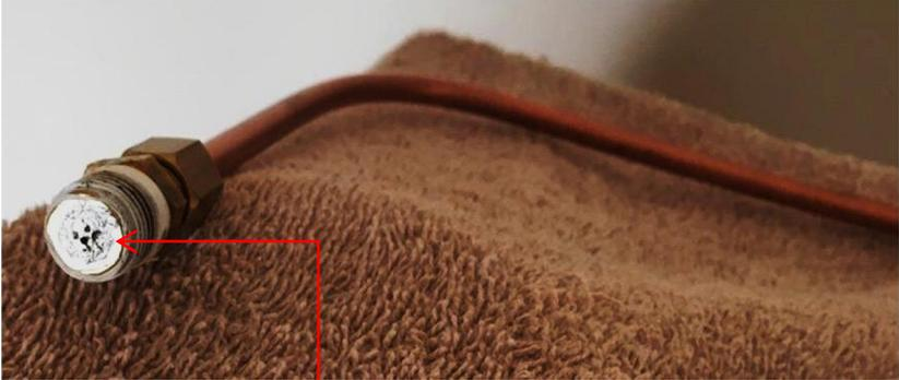
Very carefully clean out the tiny hole with a needle. DO NOT MAKE IT BIGGER, just gently clean it
