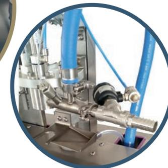
**OTHER ADVANTAGES:** use of self priming rubber impeller pump with bypass and total draining valve; filling hot liquid up to 90 C° with temperature control; adjustment of filler head; inclined steel trolley; multilingual display; adjustable support for cartoon; use of pouch-up bags-cheertainer bag.
