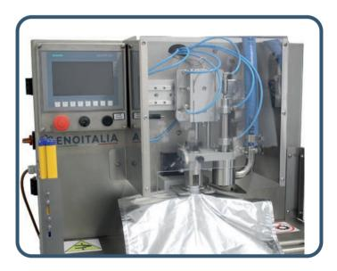
OTHER BENEFITS: large inox desk with sliding rollers and adjustable support for cardboard box; drops buffer with total drain; use of self-priming volumetric pumps with bypass and total drain valve; 7 "display; multilingual programming; oiless silenced compressor (optional).
