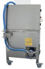
ACCURACY: The PLC SIEMENS allows to manage all phases of filling, adapting the machine to any type of treated liquid (wine, juice, oil, water, cream, etc. ..). The autotuning function allows the calibration of the machine automatically, eliminating the need to perform numerous samples. Repeatability volumes with an error of  $\pm 0.5/0.2\%$ .
