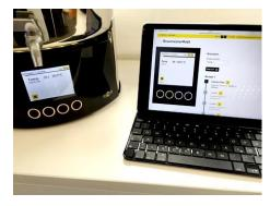
Entering the IP address into the browser address line calls up the monitoring software over the Internet and, with some delay, loads the data from the controller.
