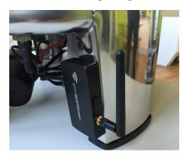
Remove the WIFI module from the protective carton and mount it on a Braumeister base. Plug the cable gland into the free socket on the reverse side of the Braumeister controller and tighten (connect the temperature sensor as well).
