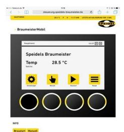
An image of the Braumeister controller is displayed. You can intervene in a controlled manner by starting a recipe, or manually, by turning the heater and pump on/off. Making settings, processing recipes and selecting temperatures needs to be performed manually on the device. In an emergency, the programme can also be stopped and terminated online.
