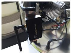
Remove the WIFI module from the carton and clip the module to the side-base on the Braumeister using the clamp on the reverse side of the module. In the beginning, this type of clamp is always very stiff, in order to make sure that module remains tightly clamped to the base. The module is clamped to the side of the controller on the 2001 and 5001 operating models. On the reverse side of the controller on the new 2015 generation, you will find another screw connector next
