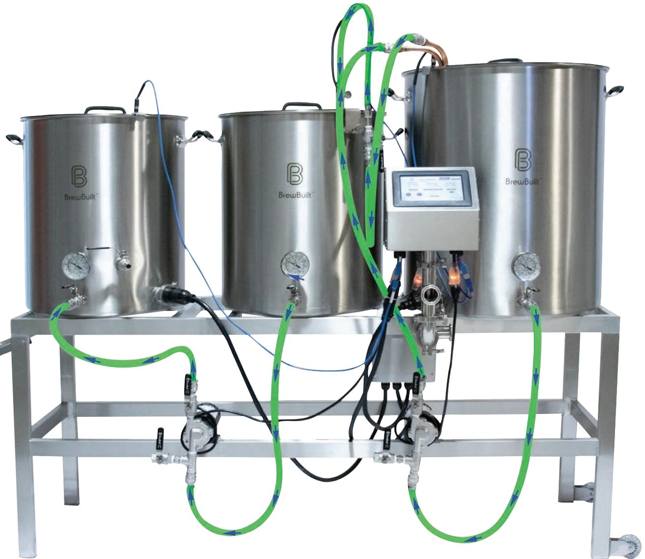
If you set the power slider on the Sparge Screen to 50% it will keep your HLT warm while preheating the boil. It will not turn on the boil element till the float switch reads UP and it will kill the HLT element when the HLT float reads DN.
