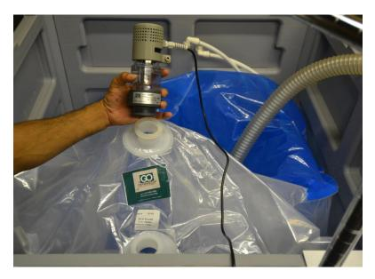
6. Use the supplied suspension cord to hang the VENT VALVE from the support pole located on the left side of the GOFERMENTOR control panel. The keeps the VENT assembly from falling into the GOBASE. Adjust the cord so that VENT assembly is above the lip of the outer container.
