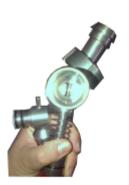
Acting on the locking screws n  $^{\circ}$  B Figure 5, it is possible to complete disassembly filling head so you can immerse in a detergent solution / sanitized, and remove all encrustations. Even in this case, be sure to keep open the filling heads to about 20mm.
