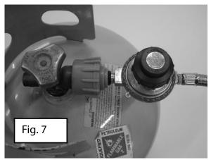
To ignite the burner, start with the damper about 1/3 open. Place a long match or igniter through the flame inspection hole, then turn the regulator slowly clockwise until you hear the gas flowing and the flame ignites.
