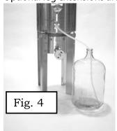
**Danger:** Do not exceed 175lb (about a 30 gal kettle) when using the leg extensions.
