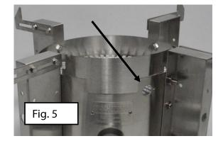
**Igniting the burner:** Always use a long match or igniter to light the burners. Never light the burner at the venturi. An ignition/flame inspection hole (Fig 5) has been provided for this purpose.
