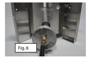
Make sure you ignite the burner with a kettle on the burner and make sure it at least partially full of water to prevent damaging the pot. A variable pressure regulator (0-10 PSI) has been provided with the stand – ref Fig 7. Turn it fully counterclockwise to the "off" position. Then turn on the tank valve to the full on position. You will use the regulator to control the gas flow and power level of the burner by turning it clockwise to increase fuel flow.
