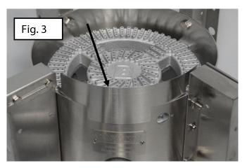
The HellFire burner includes the patent pending heat shield as shown in Fig 3. This heat shield is intended to shield the ancillary equipment mounted to the kettle such as the valve, thermometer and level gauge. However, the user must ensure that during operation all equipment is operated in its intended temperature range.
