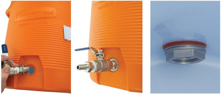
**Step Six** — At this point, you will want to use a set of crescent wrenches (3) to tighten down on the bulkhead (4a) and lock nut (4d), ensuring a leak proof seal! **NOTE:** We recommend filling your cooler with cool water before first-time use, to confirm that the bulkhead is tight and does not leak! If leaking occurs, tighten down the bulkhead until it doesn't!
