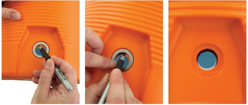
**Step Four** — Using a general purpose half-round file (1), begin to slowly expand the traced spigot hole. **NOTE:** Be careful to not file out too much, as going outside of the template will result in a non-sealing spigot!
