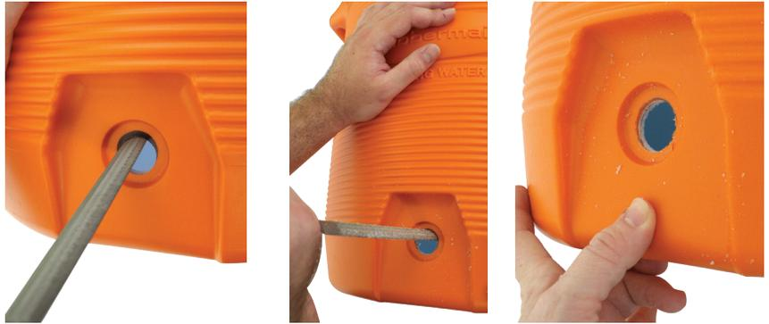
**Step Five** — Once the hole is filed out and cleaned of debris, push your bulkhead (4a) through the newly expanded spigot hole on the outside of the cooler. On the inside of the cooler, replace the red gasket (4b), then the stainless washer (4c), and finally, thread the lock nut (4d) onto the bulkhead, sealing the system.
