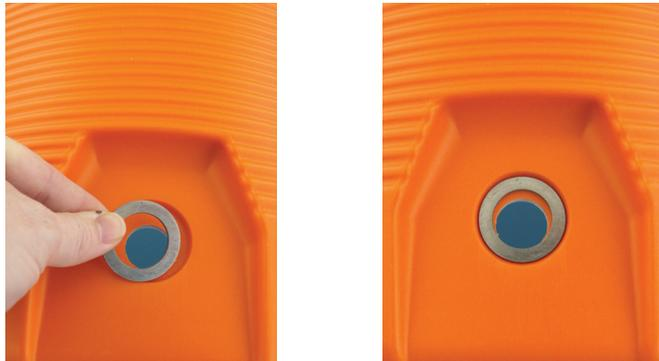
**Step Three** — Using a black felt tip pen (2), trace inside the stainless washer (4c), creating a template for filing out the hole. When you are done tracing you will have what looks like a crescent moon shape (see far right image).
