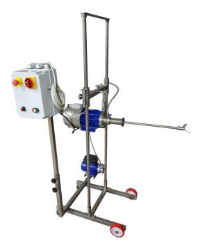
The machine is provided complete with inox trolley, where the control panel is installed with the following buttons:
