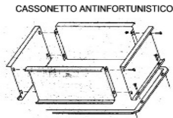
System to fix the upper safety box
