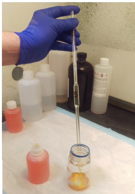
Figure 9. Delivering the Oxidant to the Reaction bottle. Touch the tip of the pipette to the side of the bottle to get complete, reproducible delivery.
