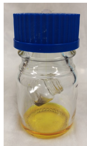
Figure 2. The ABV Reaction bottle assembly. The sample is suspended above the Oxidant in a small vial (the “bucket”), so only volatile components (ethanol) can react.
