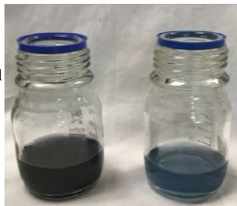
Figure 5. Titration near endpoint after addition of starch (L), and at endpoint (R).
