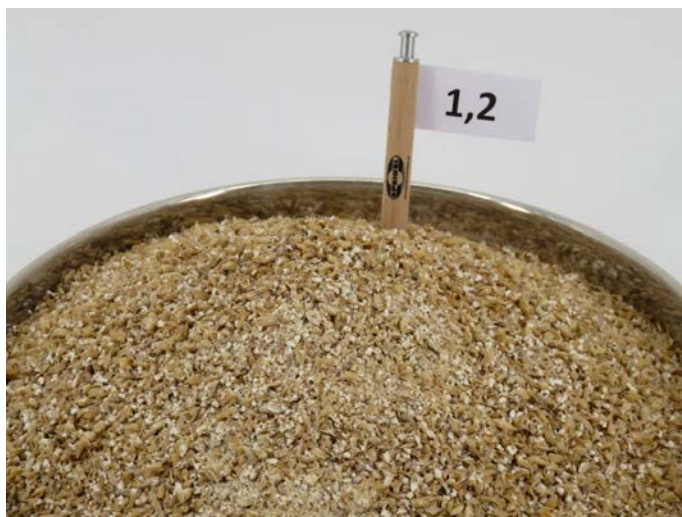
Clearance of 1.2 mm; clearly too finely grinded.
