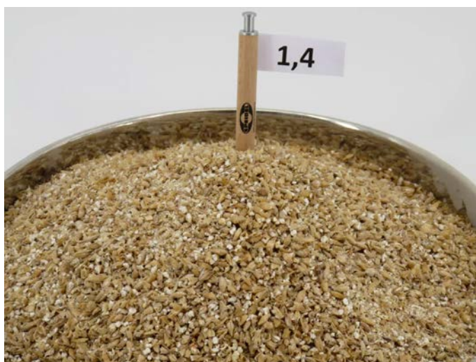
Clearance of 1.4 mm; not yet completely optimal.
