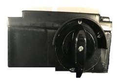
On EURO 20-30-40-50-60 coaxial models with integrated electrical panel, the pump has an inverter installed on the electric motor. In addition to the stop position "0" on the rotation inverter, position 1 (clockwise rotation) and position 2 (counter clockwise rotation) are also indicated.
