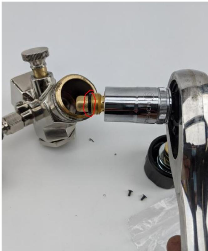
Replace the brass seat and seat cap assembly with a new one. Ensure that you adequately tighten this seat cap assembly and then re-assemble the regulator in the reverse order.
