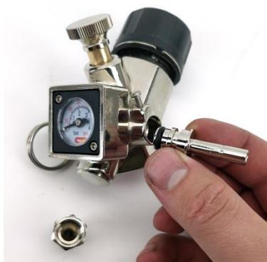
Insert required fitting into desired output and retighten grub screw
