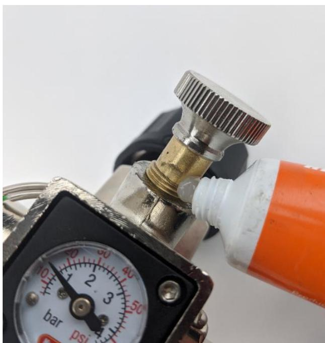
**NOTE:** It is perfectly normal for the thumb screw to be tight when under pressure. When the regulator has a cylinder attached and is under pressure it is completely normal for the thumb screw to be more difficult to turn but with moderate force it still will move. When the pressure is released it will become easier to turn.
