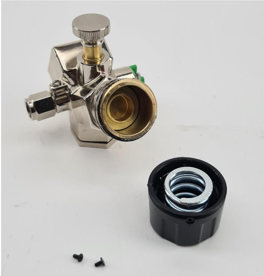
**Step 3.** Using a set of needle nose pliers remove the piston diaphragm:
