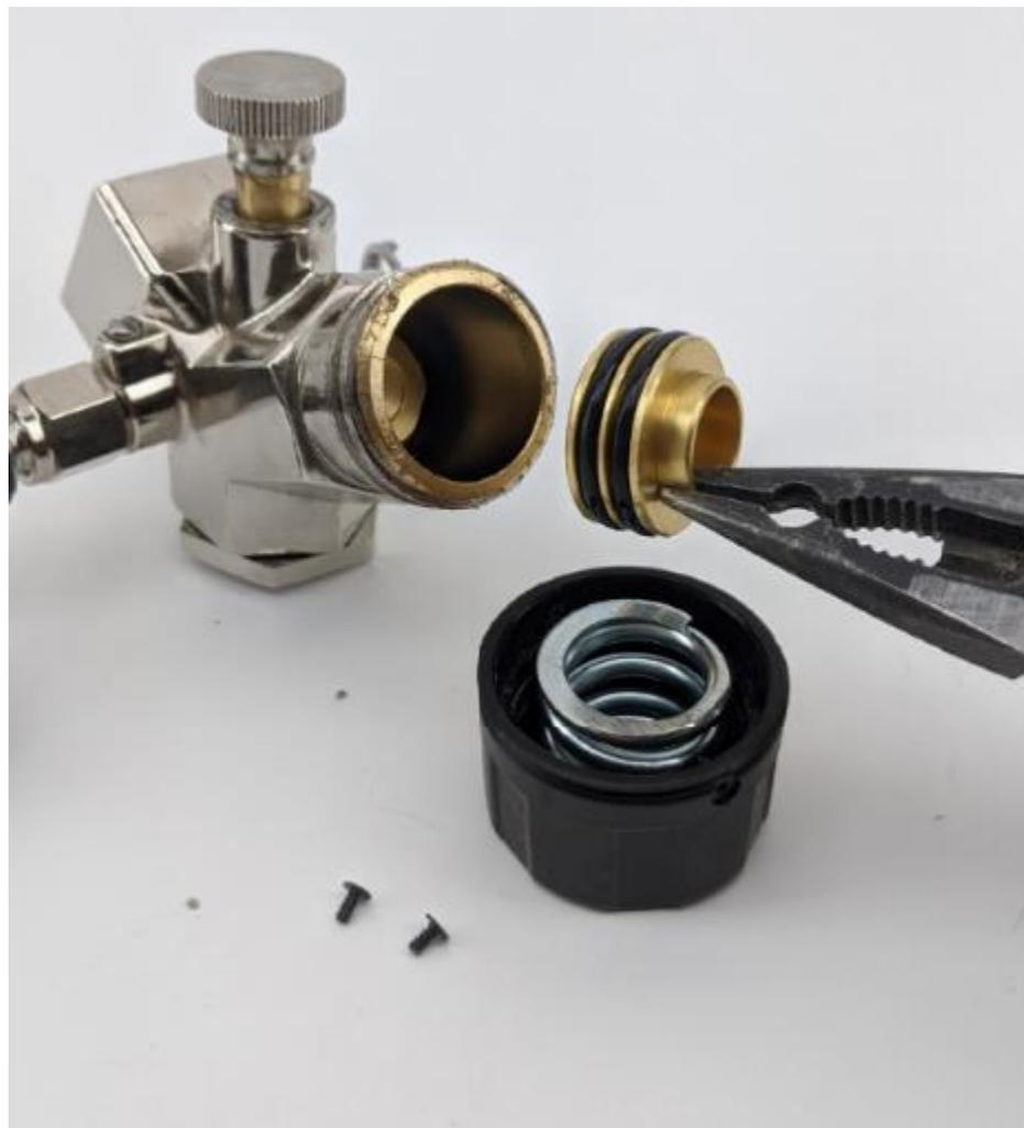
**Step 4.** With a 16mm or 5/8" socket set remove the seat and seat cap assembly. Please ensure the black o-ring comes out with this assembly. If the o-ring doesn't come out at the same time you may have to remove the o-ring separately with a pointy object:
