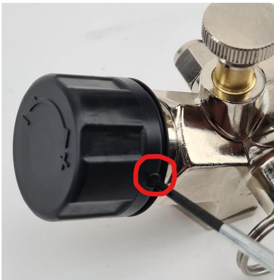
**Step 2.** Once these grub screws have been removed the regulator black knob can be completely undone and removed as shown below:
