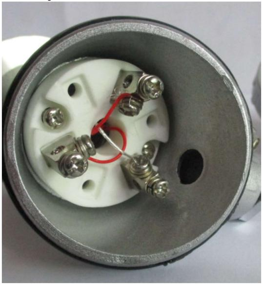
A PT100 is a positive resistance thermocouple. As the temperature increases the resistance of the thermal couple increases linearly. A resistance of 100 ohms is 32F or 0C. A resistance of 138.5 ohms is 212F or 100C.
