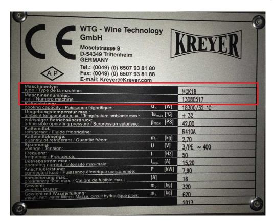
In case of technical questions or problems please <u>always</u> indicate the machine type and its serial number - see red box in the picture above! You will find this information on the type plate mounted on the outer side of each machine.
