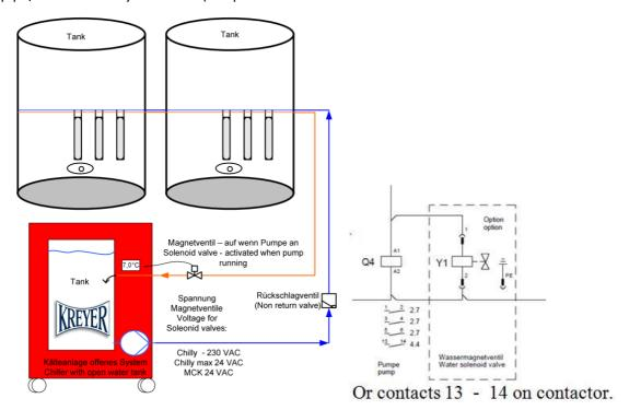
Insert the solenoid connection cable in the free cable inlet at the back side of the chiller and lead it through to the control cabinet:
