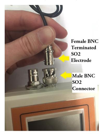
Our most current SO2 connection type. This connection type eliminates any possible issues with regards to connectivity, while also being different enough from our pH connection port so that there is no way to attach electrodes to the incorrect port.
