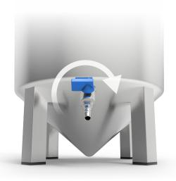
The ball valve is designed to rotate during wort transfer, which allows the racking arm to extend into the conical bottom, thus enabling you to transfer the maximum amount of beer possible. However, bear in mind that the ball valve should always be rotated clockwise, as this will prevent the valve's locknut from loosening.
