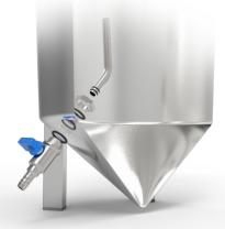
**Racking Arm**: The racking arm inserts directly into the ball valve, and is held in place by the O-rings. We recommend that you orientate the valve as shown, so that the racking arm aligns with the blue lever. This way you will know the orientation of the arm when it is submerged.
