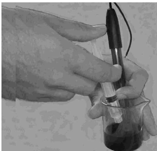
Figure 2. Manual stirring technique. Hold the electrode against the side of the vessel and swirl gently; add titrant with other hand.
