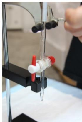
**Figure 9.** Use the end of the Electrode Holder as a guide for the glass burette for accurate titrations.
