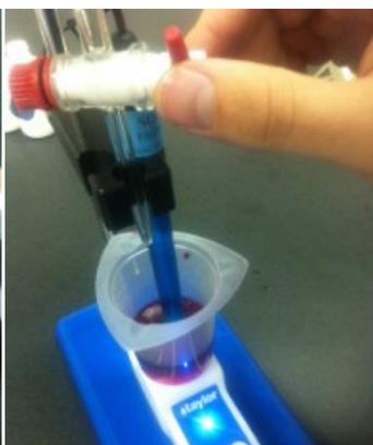
**Figure 18.** Automated stirring technique. Turn on the magnetic stirrer; add SO<sub>2</sub> Titrant by slowly opening the burette stopcock valve.
