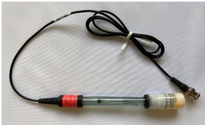
2. They have a removable sensor protector. This can be unscrewed to better access the vicinity of the glass bulb (pH sensor) for cleaning. However, you do not want to clean the glass bulb itself by physical contact in any way – contact us if you have questions. Don't try to use the electrode without its protector in place – the glass bulb is very fragile.
