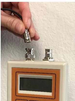
**Figure 2.** Attach the SO<sub>2</sub> electrode to the connector on the SC-300.
