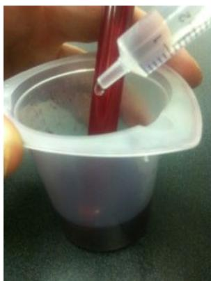
**Figure 21.** Manual stirring technique. Hold the electrode against the side of the titration beaker and swirl gently; add TA Titrant with other hand.
