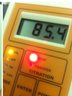
**Figure 20.** Once the device beeps for 15 seconds or 20 sets of "beep-beep" you are done with the titration. The red "STOP" LED will also remain lit.
