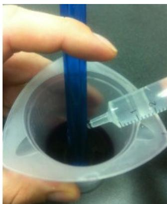
**Figure 17.** Manual stirring technique. Hold the electrode against the side of the titration beaker and swirl gently; add SO<sub>2</sub> Titrant with other hand.
