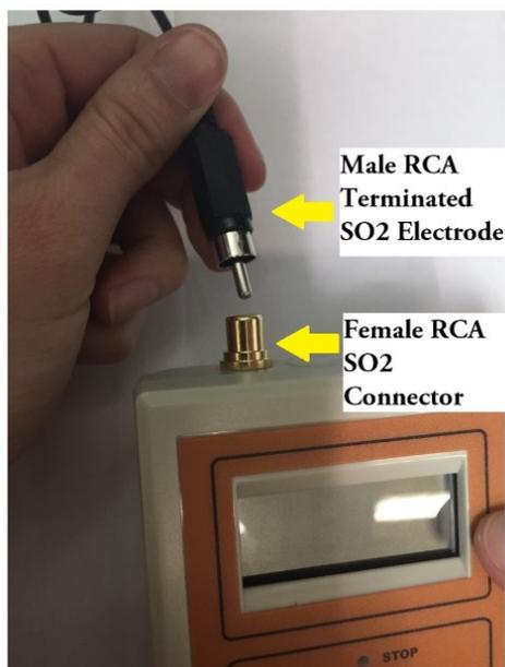
3. The platinum wires of your SO<sub>2</sub> electrode could be dirty (crust, debris, etc.) even though you may not be able to see anything. First, soak the SO<sub>2</sub> electrode in your Acid Solution for about 10 minutes and rinse with DI water. Using the back edge of a pocket knife or something similar, very gently scrape the two platinum wires, being sure not to bend or break them. Thoroughly rinse with DI water and try your test again.
