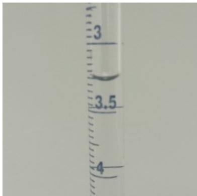
**Figure 12.** The meniscus of the water column. We recommend measuring the titrant volume from the bottom of the meniscus. In the picture the value is about 3.27 mL.
