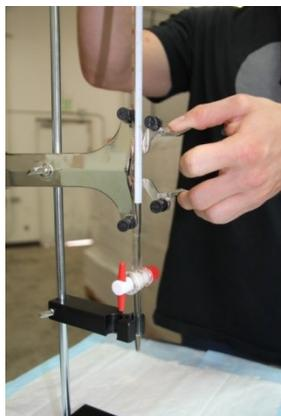
**Figure 8.** The burette sits firmly between the notches of the four spring arm knobs of the Double Burette Clamp.
