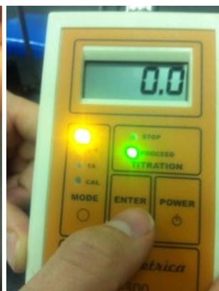
**Figure 19.** Make sure that the "PROCEED" LED is lit. You should be reading close to 0.0 when you first start. You are now ready to titrate!
