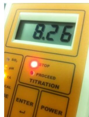
**Figure 24.** Once the pH arrives at or passes 8.20 you are done with the titration. The red "STOP" LED will be lit and the instrument will be beeping
