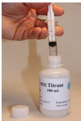
**Figure 14.** Withdraw the titrant from its bottle using a clean 5 mL syringe. If you are using the glass burette, use the syringe to fill it.
