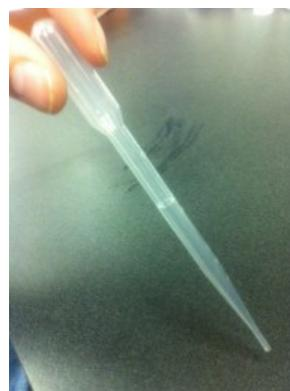
**Figure 16.** The transfer pipette. One full squeeze of the transfer pipette in either the Acid solution or Reactant should be approximately 2 mL.
