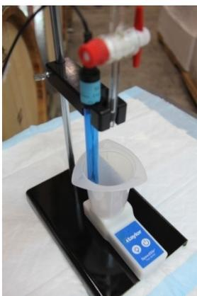
**Figure 4.** The Magnetic stirrer and beaker with the pH electrode inserted into the Electrode Holder to the wine sample.
