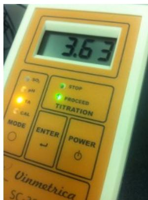
**Figure 23.** Make sure that the green "PROCEED" LED is lit. You should be reading a pH close to what you expect your wine is at. You are ready to titrate!
