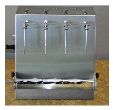
2.2 Unscrew the fixation screws holding the shelf to the machine body, and move the shelf to the bottom of the machine. Plug the electrical connector into the side of the filler (shown with optional gas sparge).
