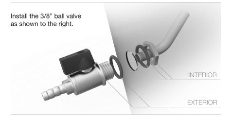
You only need to get the retaining nut for the ball valve / racking arm assembly **finger tight** so that the assembly can rotate clockwise at least a half turn. **Do not** use a wrench.
