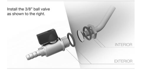
You only need to get the retaining nut for the ball valve / racking arm assembly **finger tight** so that the assembly can rotate clockwise at least a half turn. **Do not** use a wrench.
