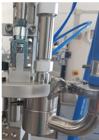
Non-drip head, standard with olive oil kit installation and hot liquid filling
