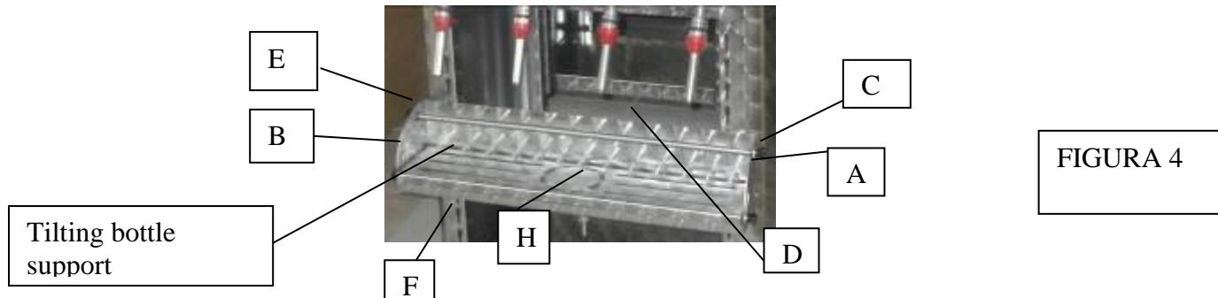
Once settle the desired level, place the bottle in vertical and lift the support surface of the bottles (use the F holes for adjustment), going to install it in a location as close as possible to the bottom of the bottle (the surface of the support must be parallel and not tilted).
