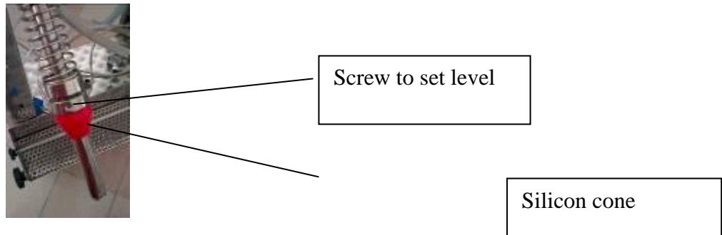
Place the bottle you want to fill inside a filling head, while touching the mouth of the bottle to the silicon cone. Not to push the bottle upwards.
