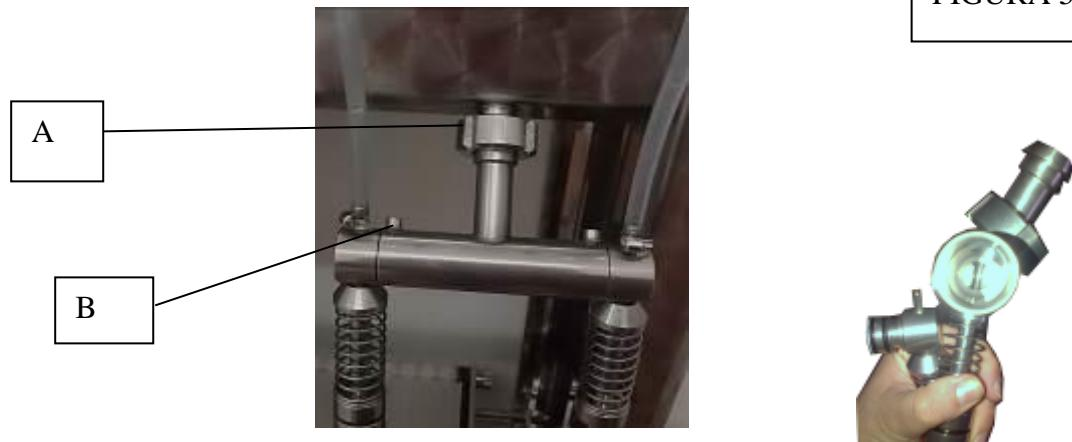
Acting on the locking screws n ° B Figure 5, it is possible to complete disassembly filling head so you can immerse in a detergent solution / sanitized, and remove all encrustations. Even in this case, be sure to keep open the filling heads to about 20mm.
